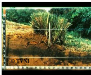
Cross section showing a 60 cm terrace formation, which formed over 2.5 years.
